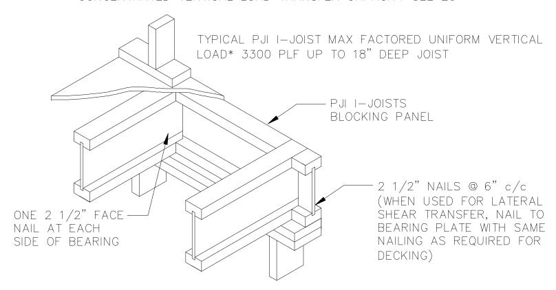
TO AVOID SPLITTING FLANGES , START NAILS 1  $\frac{1}{2}$ " FROM END OF I-JOIST. NAILS MAY BE DRIVEN IN AT AN ANGLE TO AVOID SPLITING BEARING PLATE
