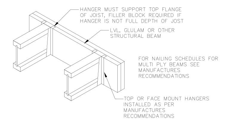
ALL NAILS SHOWN IN THESE DETAILS TO BE COMMON NAILS UNLESS OTHERWISE NOTED. 3" BOX MAILS MAY BE SUBSTITUTED FOR 2 1/2" COMMON NAILS
