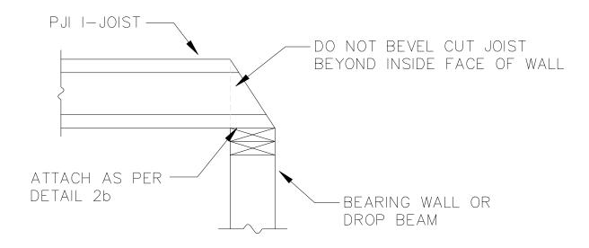
NOTE: BLOCKING REQUIRED AT BEARING SUPPORT. NOT SHOWN FOR CLARITY
