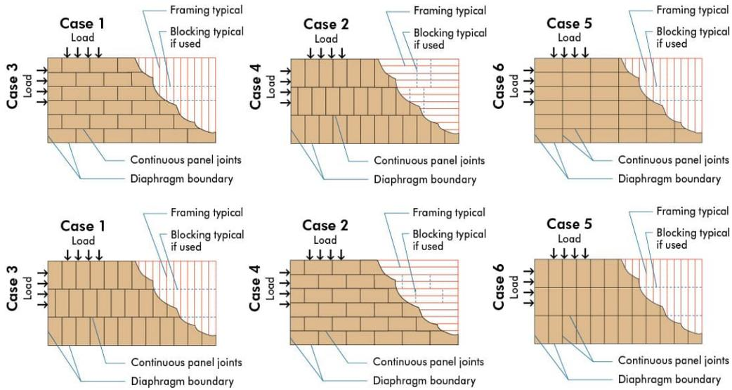
Figure 1. Diaphragm configurations
