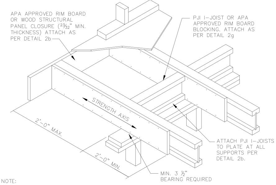
MIN. 23/32" THICK APA SPAN RATED SHEATHING 48/24 OSB REQUIRED ON SIDE OF JOIST. DEPTH SHALL MATCH FULL HEIGHT OF JOIST. NAIL BOTH TOP AND BOTTOM FLANGES w/ 2 1/2" NAILS @ 6"c/c. INSTALL WITH STRENGTH AXIS HORIZONTAL AS SHOWN. ATTACH PJI TO PLATE AS PER DETAIL 2b
