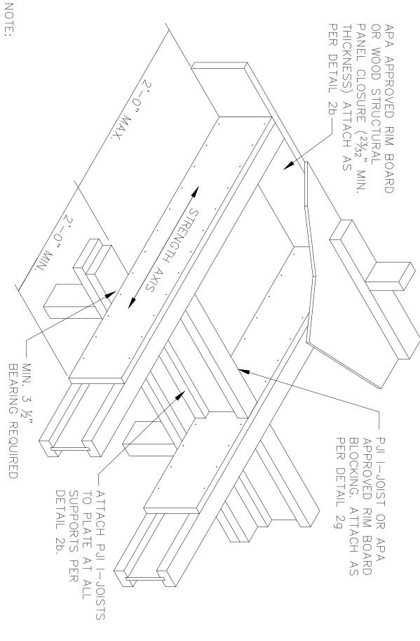
SHALL MATCH FULL HEIGHT OF JOIST. NAIL BOTH TOP AND BOTTOM FLANGES INSTALL WITH STRENGTH AXIS HORIZONTAL AS SHOWN. ATTACH PJI TO PLATE MIN. 23/32" THICK APA SPAN RATED SHEATHING 48/24 OSB REQUIRED 9 2 1/2" NAILS @ SIDE OF PER DETAIL 2b JOIST. DEPTH
