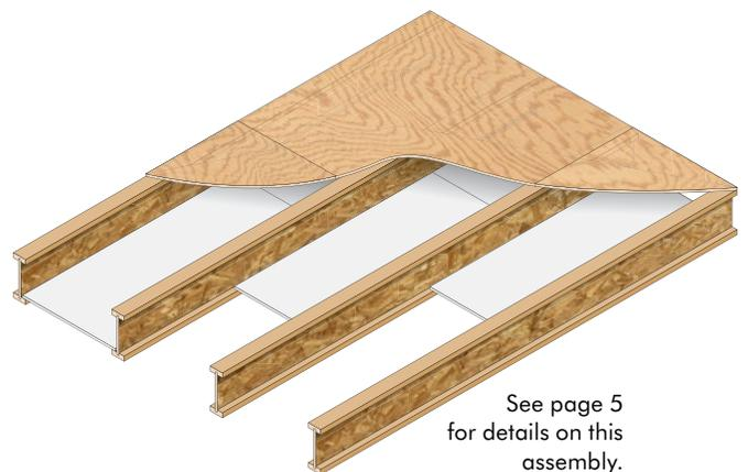
**1/2-inch Gypsum Board Installed on Top of the Bottom Flange for I-joist Spacing 19.2 inches or less on center. (FP-06 in System Report SR-405)**
