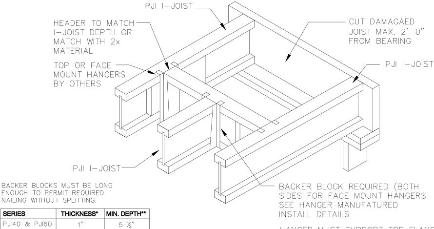
\*MIN GRADE BACKER BLOCK SHALL BE UTILITY GRADE SPF (SOUTH) OR BETTER FOR SOLID SAWN LUMBER AND SHALL BE RATED SHEATHING GRADE FOR WOOD STRUCTURAL PANELS.
